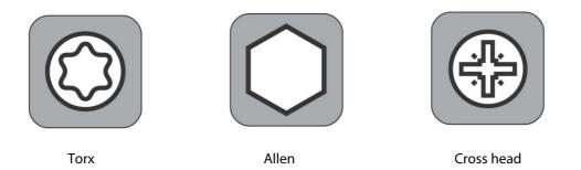
Image 8: Three types of fixing heads used
