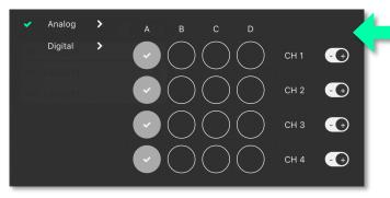
Analog CH A is routed to all outputs.
