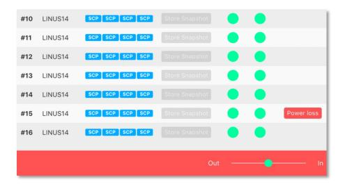
To acknowledge either condition (Error or Warning), click the "Power Loss" announcement. This changes the colour to grey & changes the Bottom Toolbar to its default black colour. When the fault clears, the "Power Loss" announcement will disappear.
