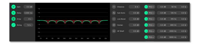
All group tuning parameters are enabled and disabled by clicking on the corresponding icon. A greyed-out icon means the parameter is disabled. A green icon means the parameter is enabled.
