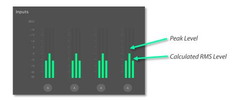
If the input meters are hitting the top (turning orange or red), and the loudspeakers are not in gain reduction, it would be wise to assess the gain structure of the system to prevent
