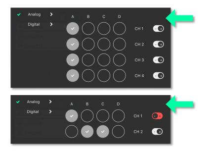
Analog CH A is routed to all outputs. All the outputs are in Polarity.
