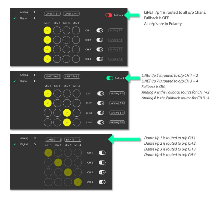
Note – The Dante patch is fixed one to one in the Firmware. To adjust the routing of the Dante, please use Audinate's Dante Controller.
