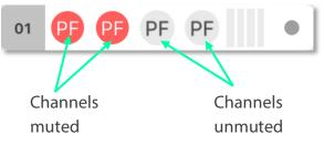
When the channel mutes are off, output meters are displayed in green behind the suffix. The output meters are calibrated in dB relative to the speakers full RMS output potential on a per-channel basis.
