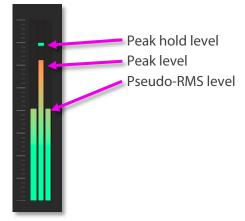
If the input meters are hitting the top (turning orange or red), and the loudspeakers are not in gain reduction, it would be wise to assess the gain structure of the system to prevent overloading or overshooting the input stage. Attenuate the input signal and increase the system gain.
