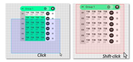
Note - A new feature within LINUS Control v2.1.18 compared to existing versions is the ability to add amplifiers to a group automatically when the group is added to the workspace. To do this, first select the amplifiers you wish the group to be in control of, then add the group to the workspace.
