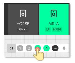
When the loudspeaker is in 'ASSIGN' mode, the channels can be selected that the loudspeaker should be assigned to.
