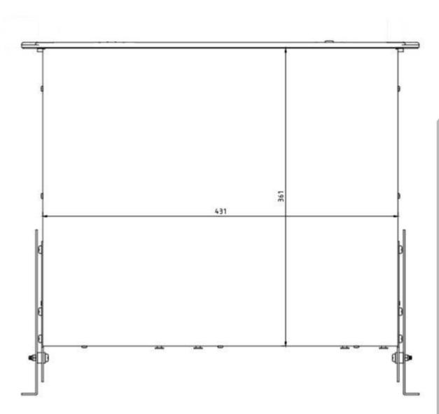
The C3 DSP amplifier system is designed to be mounted in a standard 19" rack enclosure.
