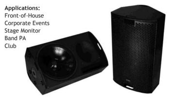
The Coda Audio K15 is a versatile, full range, two-way loudspeaker system that features a high power 15" neodymium woofer and a 1" neodymium compression driver coupled to an  $80^{\circ}$  x  $60^{\circ}$  routable elliptical waveguide.
