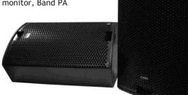
The Coda Audio Rx36 is a versatile, full range, three-way loudspeaker system that features a high power 15" neodymium woofer and a 2" coaxial neodymium driver coupled to a 60° x 40° waveguide. As a 3-way system, the Rx36 may be driven passively or with bi-amplification to provide extremely high acoustic output.
